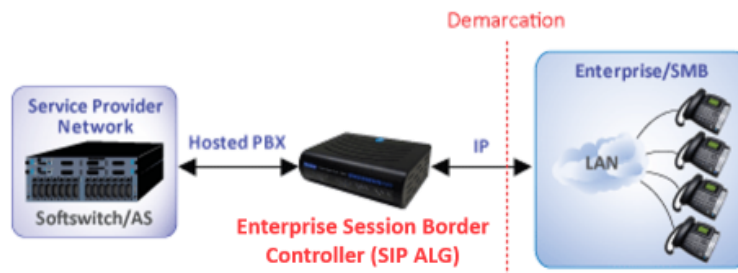
Figure 124. Hosted Voice Service delivered by the ESBC SIP-ALG module
