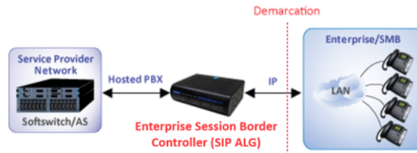
Figure 3. Hosted Service Using ESBCs with SIP ALG
