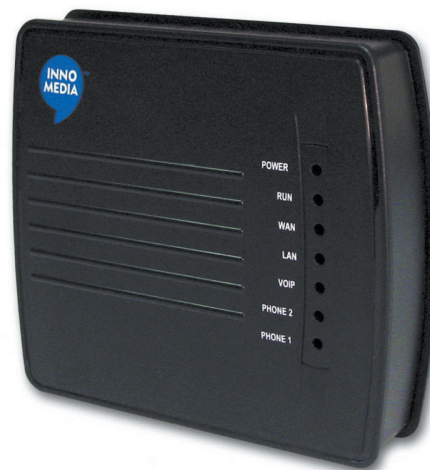
Standalone MTA 6328-2Re with 2 voice ports
